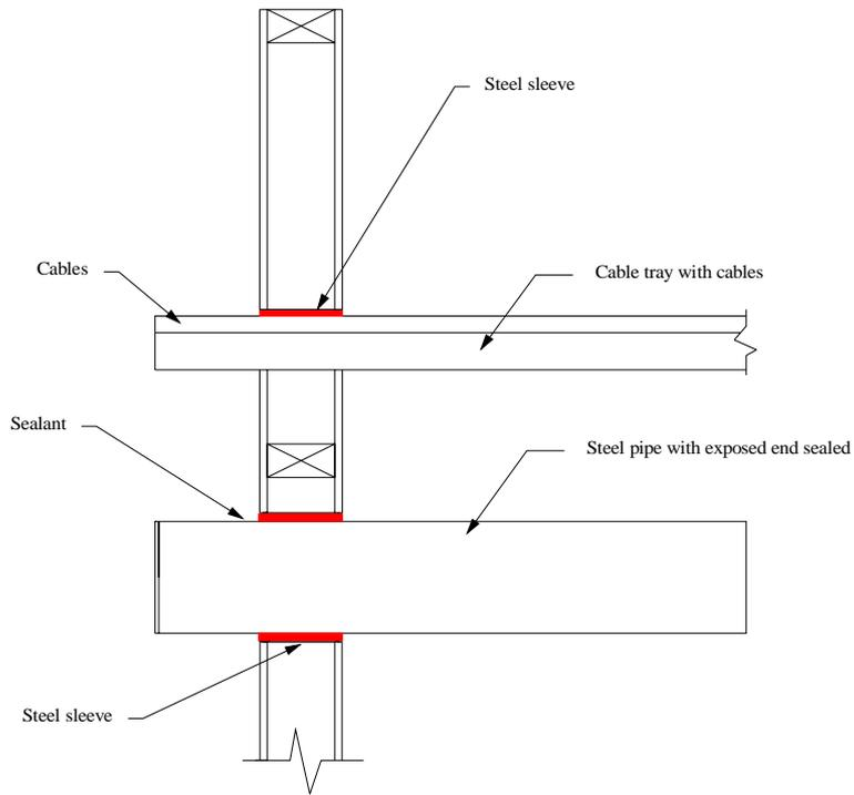
**Figure 8 Sections through penetrations**
