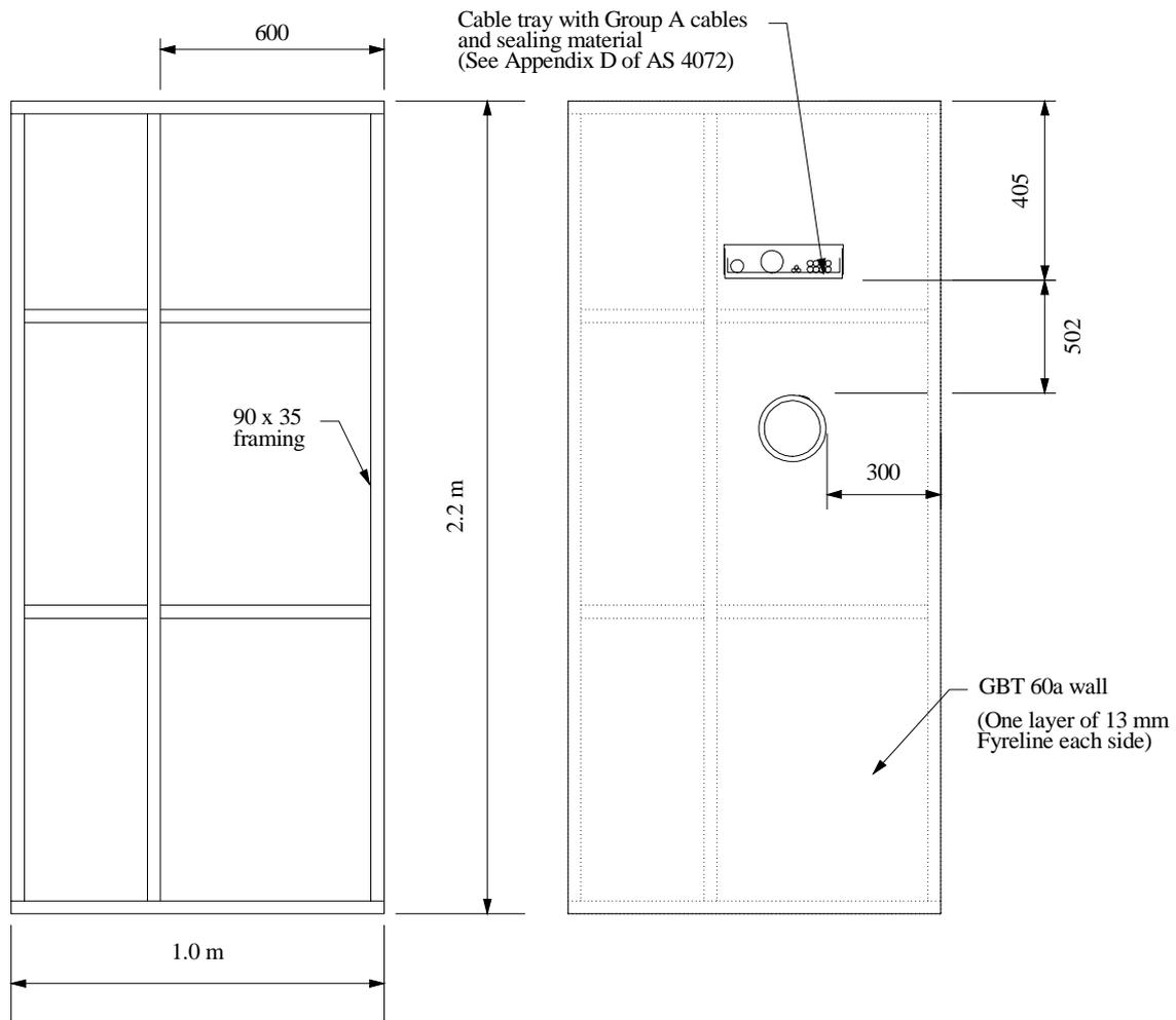
**Figure 6 Specimen Layout**
