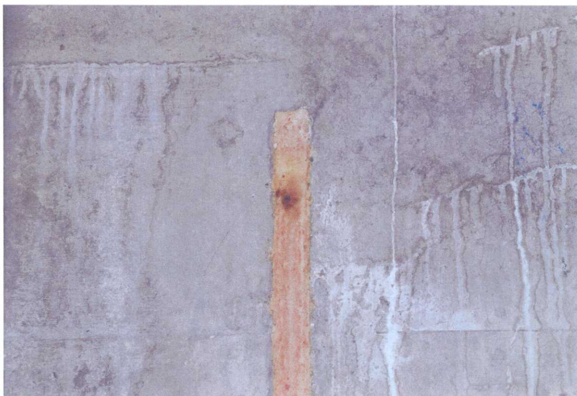
Detail of the beginning of piercing at the upper part of seal B, 30 mm, at 4 h and 51 min. of test
