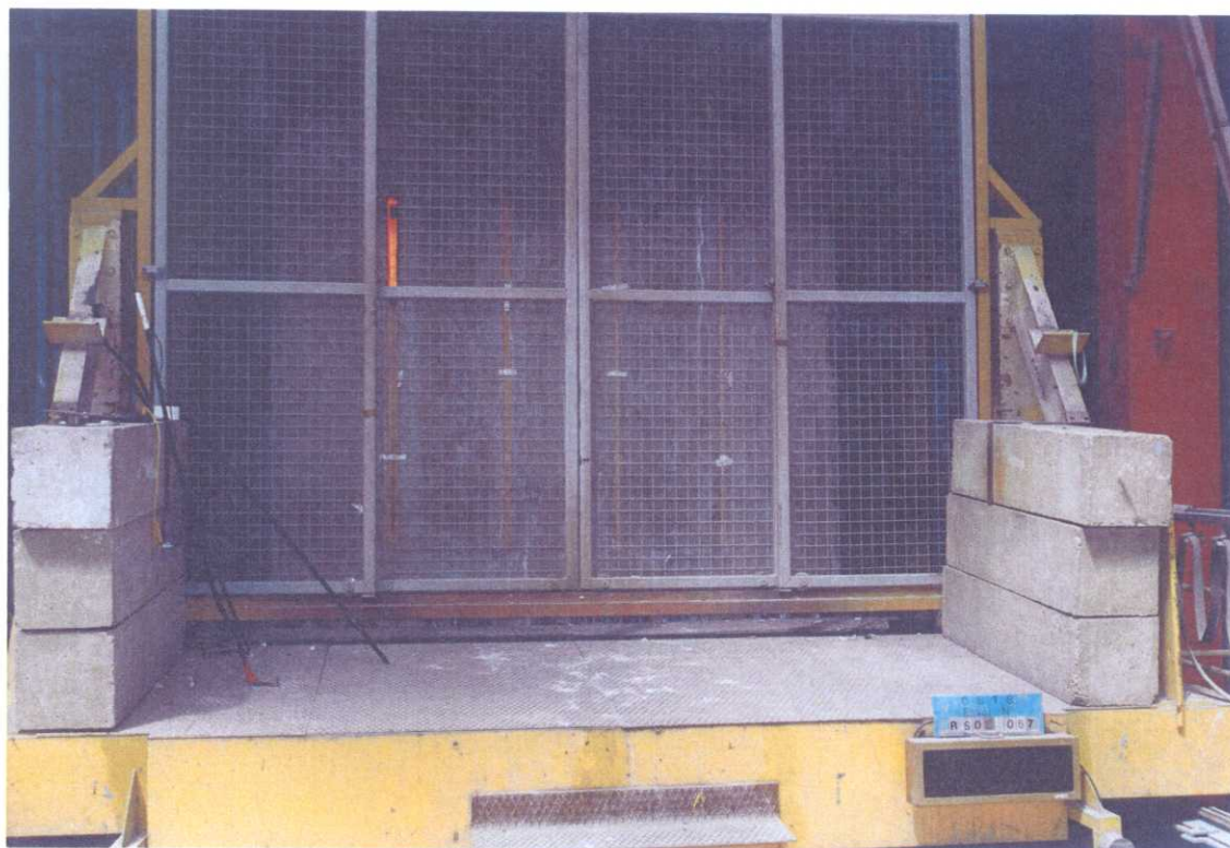
Photo of the face not exposed to the fire at 4 h of test
