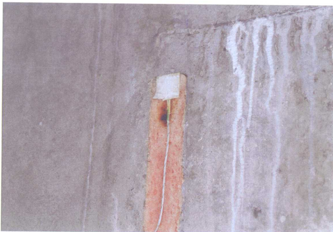
Detail of the beginning of piercing at the upper part of seal A, 40 mm, at 3 h and 38 min. of test
