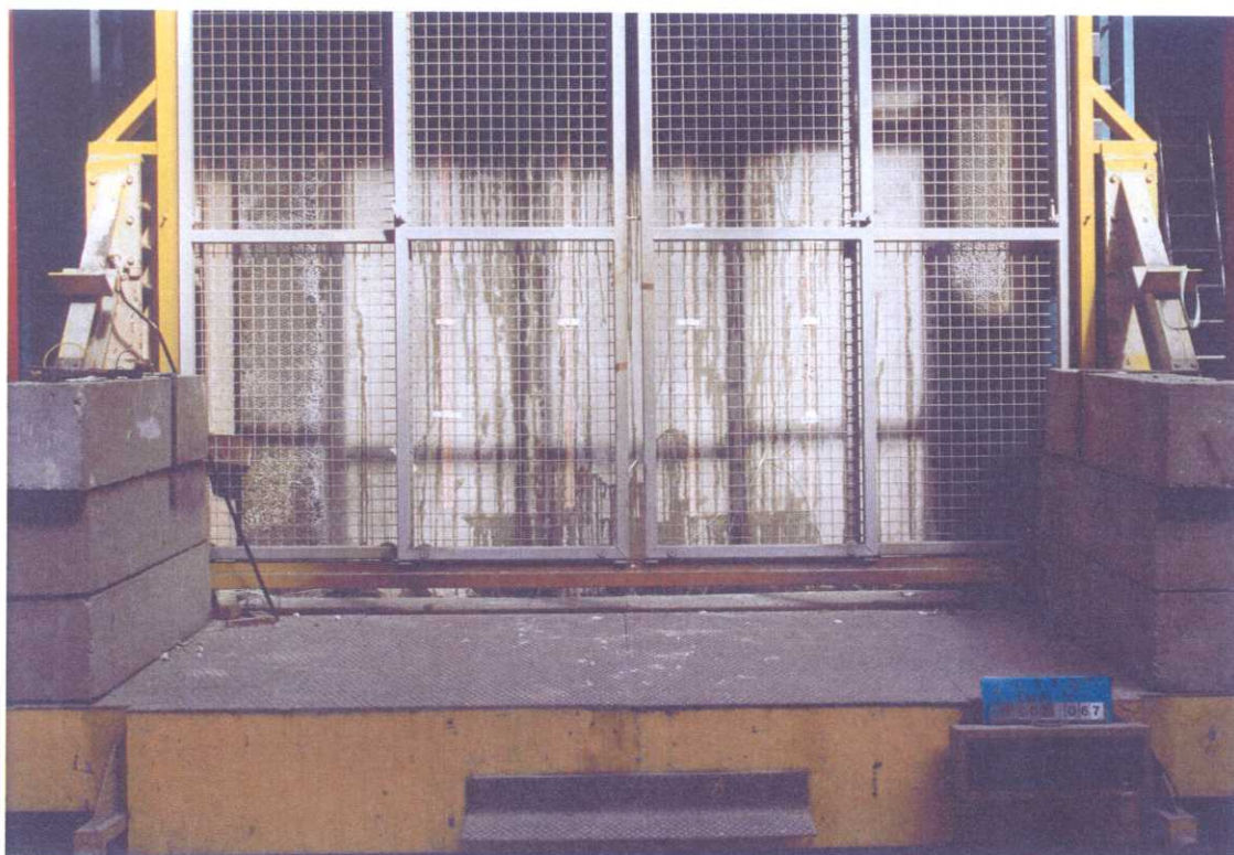
Photo of the face not exposed to the fire at 1 h of the test
