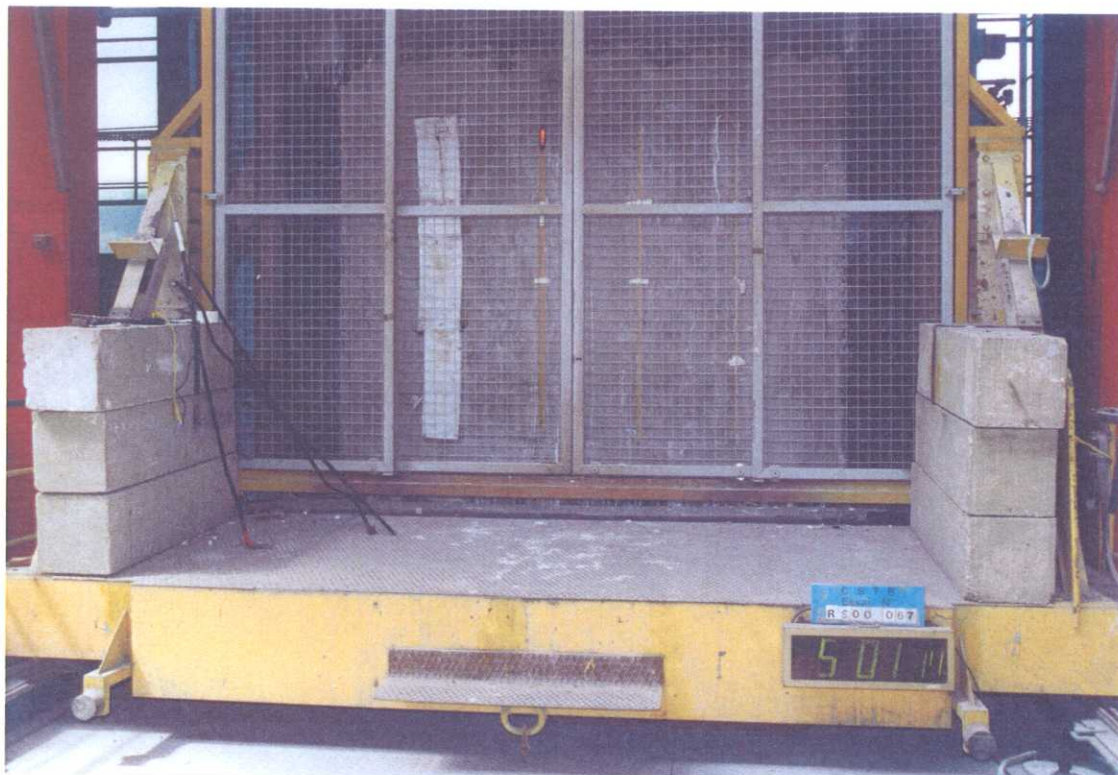
Photo of the face not exposed to the fire at 5 h of test
