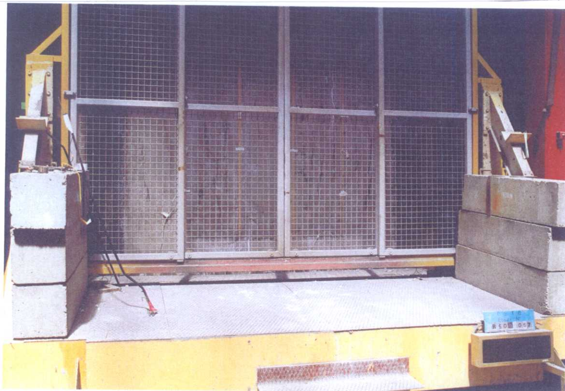
Photo of the face not exposed to the fire at 3 h of test
