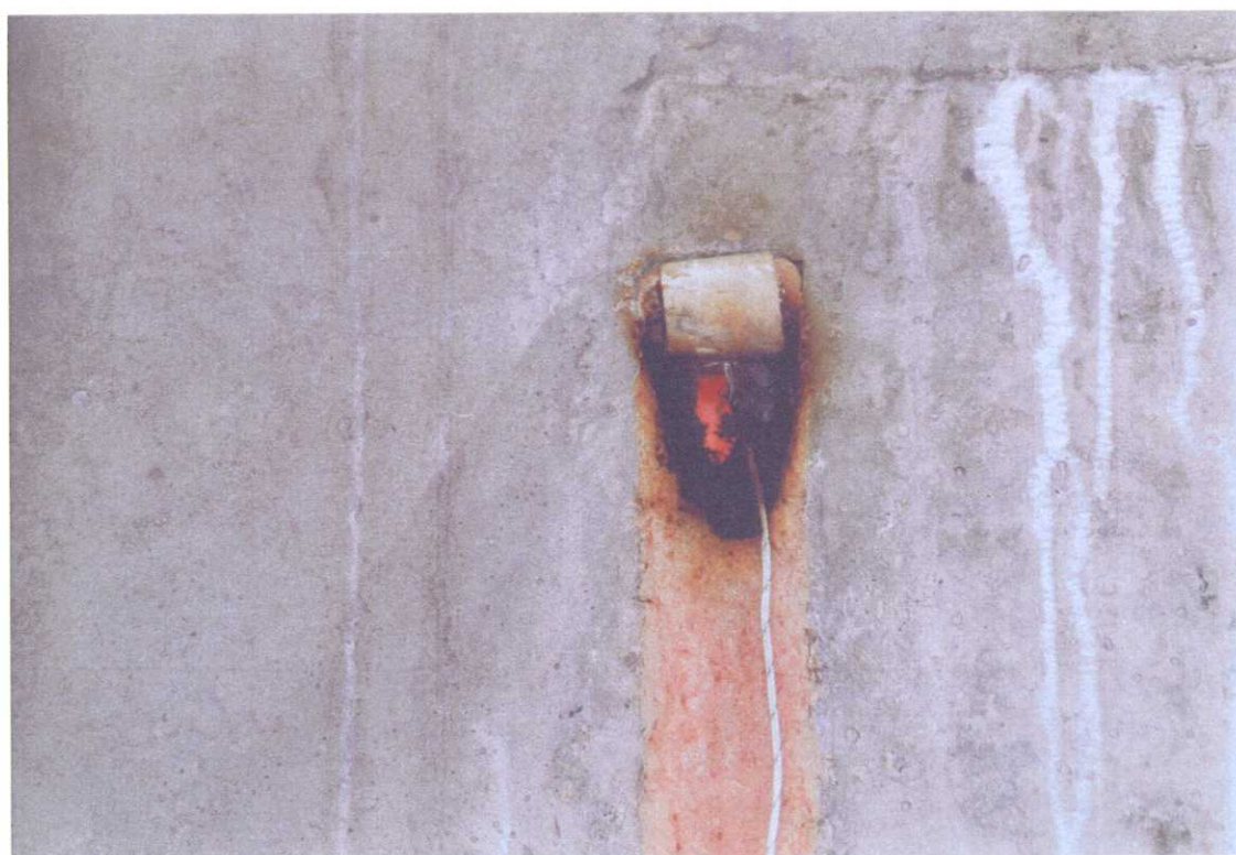
Detail of the opening at the upper part of seal A, 40 mm, at 3 h and 43 min. of test
