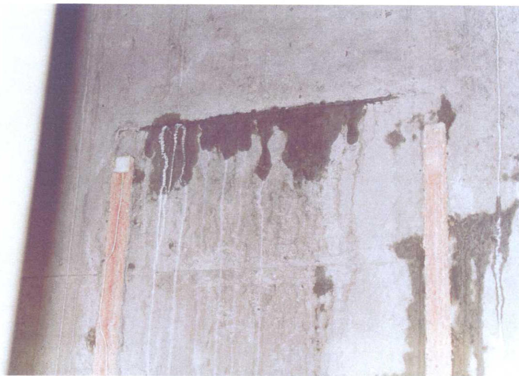
Detail of seal A, 40 mm, and seal B, 30 mm, at 2 h of test
