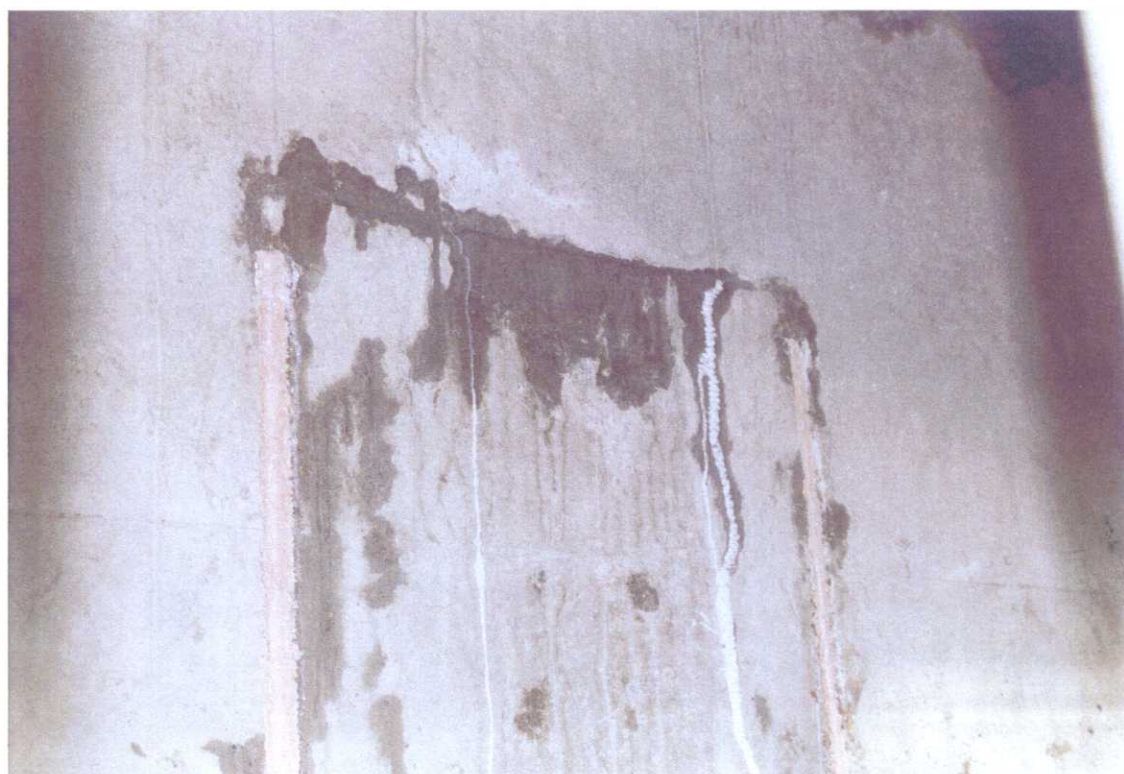
Detail of seal C, 20 mm, and seal D, 10 mm, at 2 h of test
