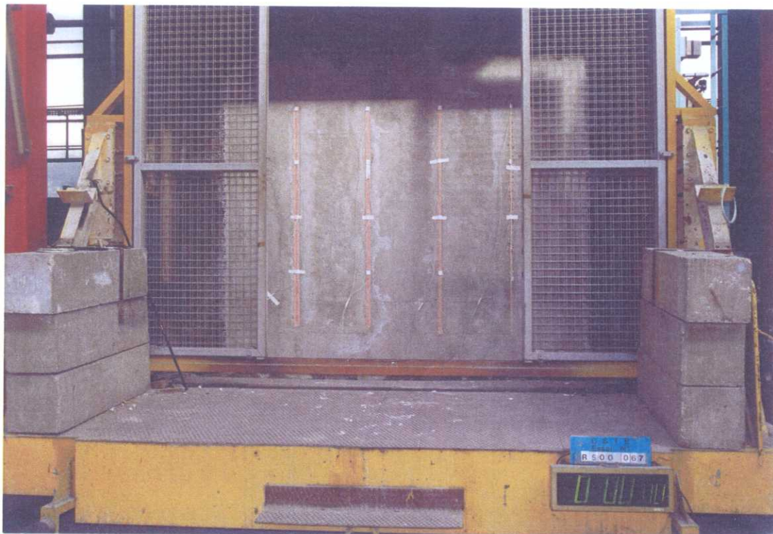
Photo of the face not exposed to the fire at the beginning of the test
