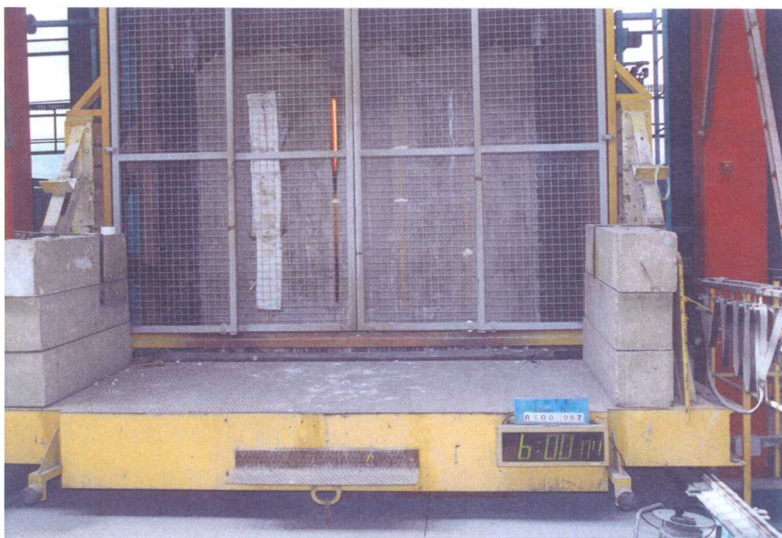
Photo of the face not exposed to fire at 6 h of test
