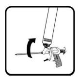
The foam can must be turned upside down for the foam to extrude.
