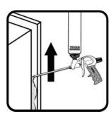
Apply foam into the joint or gap upwards, from bottom to top.
