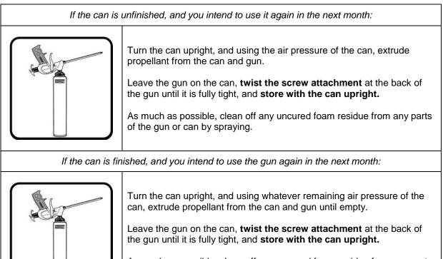
As much as possible, clean off any uncured foam residue from any parts of the gun or can by spraying.
