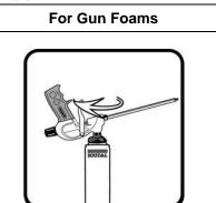
With the foam can upright, screw the foam gun onto the can.
