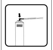
Turn the can upright, and using whatever remaining air pressure of the can, extrude propellant from the can and straw as much as possible.
