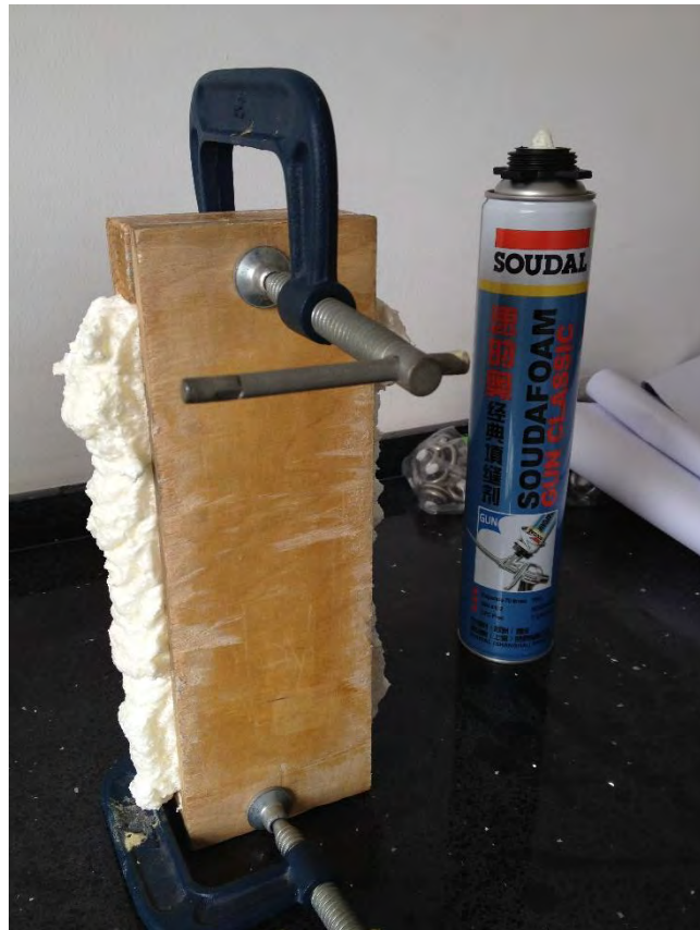
2. Foam has expanded out of the joint, two hours later.
