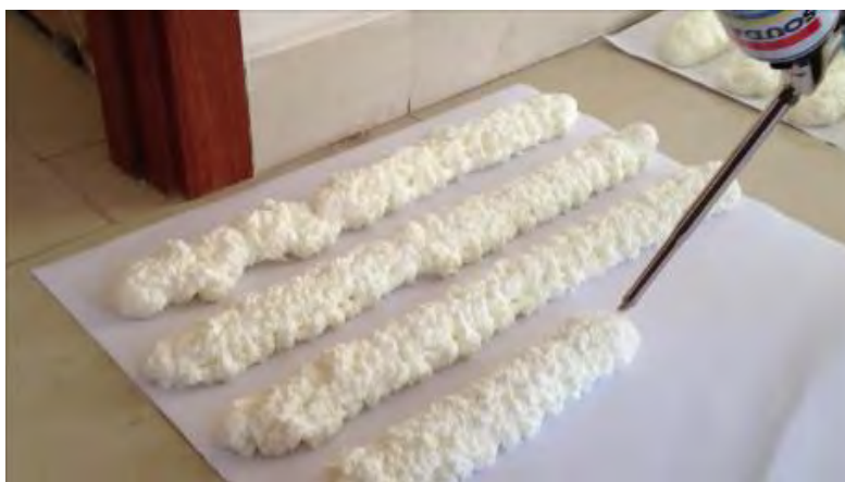
The process of extruding foam to measure the yield. This picture shows the foam before it expands to the fully cured state.
