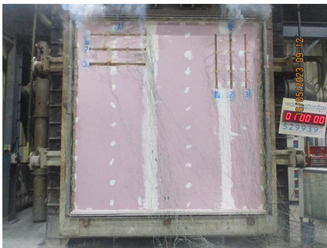
The unexposed face after a test duration of 60 minutes
